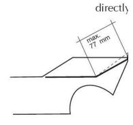
The angle to be measured over a distance of 77 mm from the highest point of the spoiler or Guerney flap to the middle of the body. You need a tool from which you can adjust the height an the angle.
