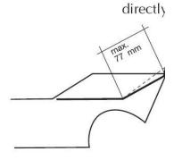
The angle to be measured over a distance of 77 mm from the highest point of the spoiler or Guerney flap to the middle of the body. You need a tool from which you can adjust the height an the angle.
